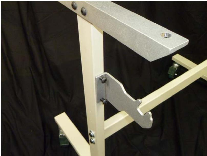
Test fit the mandrel, make sure that it fits between the mandrel brackets without the left mandrel bracket putting pressure on the mandrel, you should have a small space between the mandrel bracket and the mandrel as shown. If not, your mandrel brackets will have to be adjusted later.
