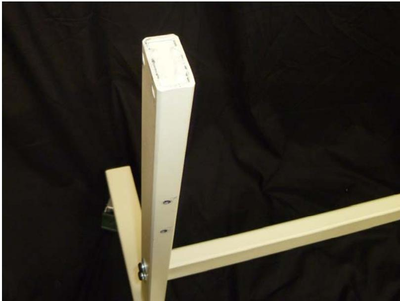
Install the machine base to the top of the riser as shown. The only orientation that matters is that the angle is mounted to the outside of the stand.
