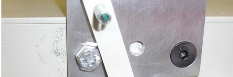
Take note that on the right tower the rear bolt must be oriented so that the side of the bolt is parallel to the side of the slitter-actuating handle (see diagram below.). Do not over tighten bolt it is better that it be looser rather than over tightened
