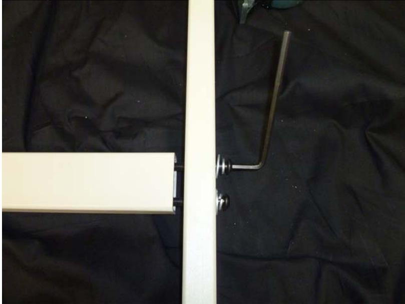
Position the now assembled sides so that the tower screws holes are located to the front. The spreader will be placed in between, you are now looking at the front of the stand.
