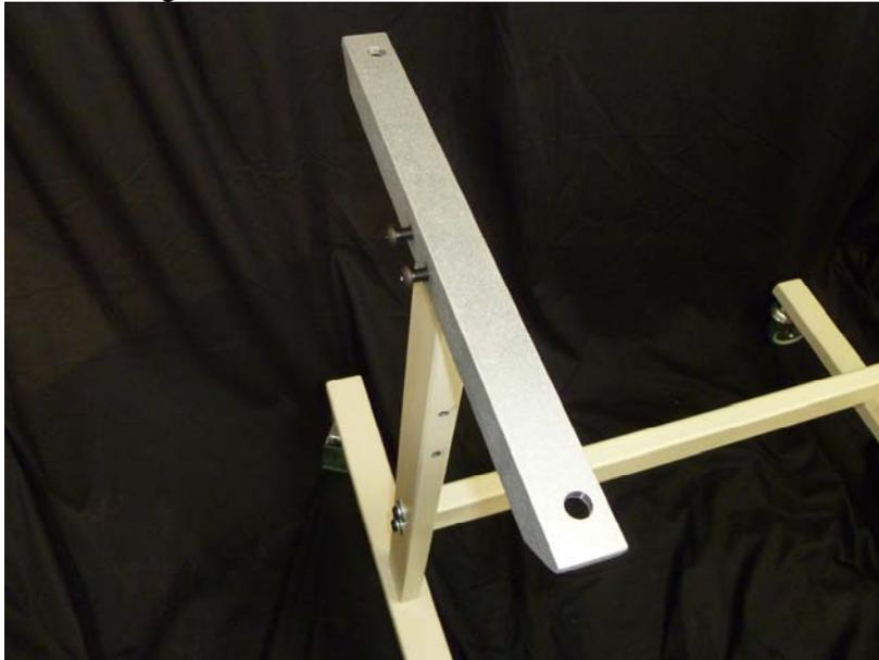
Install the other side and tighten the screws until they are snug but not tight
