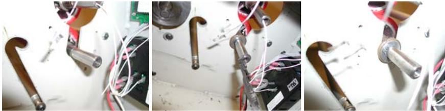
41. Install and tighten the drive sprocket, this must be measured and aligned with the other sprockets so that all of the sprockets are the same distance from the frame. Make sure when tightening the sprocket it is on the flat of the shaft (as shown) if this sprocket is poorly aligned you will notice a clicking or thumping as the machine runs.
