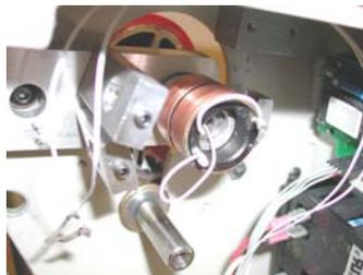
46. Check roller alignment by rotating the rollers by hand several revolutions and then check side to side alignment,
