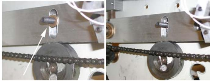
7. Loosen the motor mount screws and remove the drive chain.
