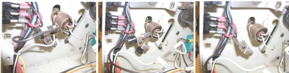
23. Remove the slip ring using a 5/64 allen wrench (similar to step 11).
