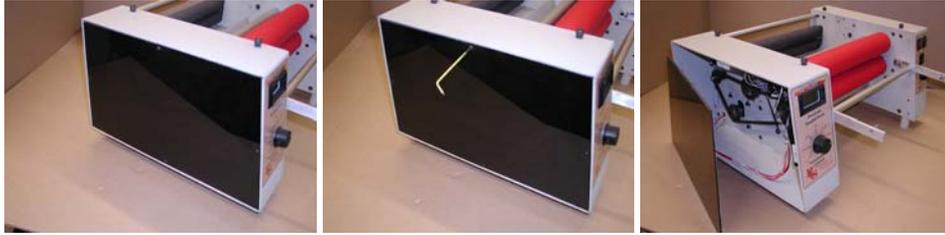
2. Remove roller-gapping handle by turning counterclockwise. This handle is located on the right side of the machine and it may require someone to hold the roller-gapping cam located under the swing in the left side panel with a large pliers. After, make sure the rollers are in the down position.
