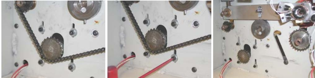
8. Unsolder the wires connected to the slip ring.
