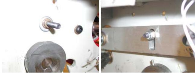
43. Install the snap ring and any spacers that were removed on the upper rear roller in step 12. Make sure snap ring is in its groove as shown in step 31
