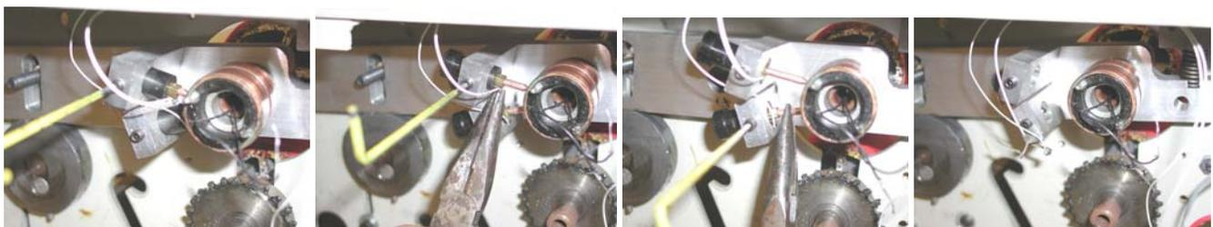
11. Loosen the set screw holding the slip ring onto the roller and remove the slip ring. You may rotate the rollers to get a better angle at the screw if necessary.
