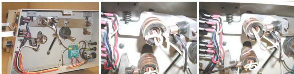
18. Remove the brushes. Loosen the set screw that holds in the brush holders partially remove the brush holder then pull out the wires from the brush holders ( they pull out do not de-solder these). (Unlike step 10. the brushes will not spring out of the front of the holder they are trapped).
