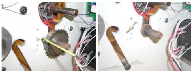
16. Remove the snap ring on the bottom heat roller (similar to step 12), do not reuse the snap ring, Remove the bronze bushing. You may need to tap the bushing out from the other side of the panel using a long screw driver and a small hammer, be careful not to damage the bushing.
