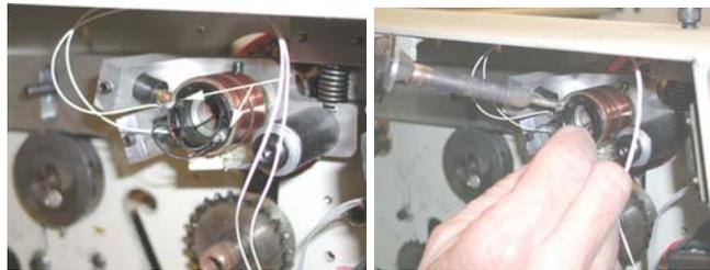
9. Remove the rubbing pad assembly. Using a 3/16 allen wrench loosen and remove the bolt.
