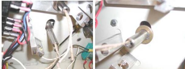
31. Install a **NEW** snap ring into the groove on the lower roller, make sure not to stretch the snap ring to far, make sure that the snap ring is completely in the groove. **If the snap ring is damaged at all during installation, make sure to replace it.** Illustration shows the proper position of the snap ring, do not install the snap ring before the roller is in the machine (the pictures below are for reference to the groove)
