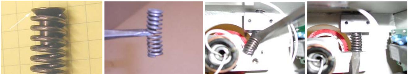
49. Install the pressure adjustment screws. Return them to their setting as recorded in step 13. The factory settings on the front roller are about 1-3 turns and on the rear rollers is 0-2 turns from the point that it starts to apply pressure to the rollers. The wider the machine the less pressure needed.
