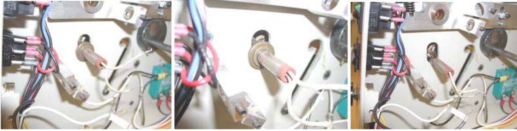
25. Remove the lower roller by lifting it up on the left then through the hole then to the left about 5" and then up on the right then out. This is the last step for removal.
