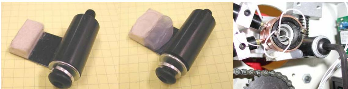
52. Install the brushes on the right side of the laminator. Install the brush wires (these wires are not polarity sensitive and may be attached to either brush holder however typically at factory the wires fit best with the black wire on the inside). Tighten only fingertip snug. Do not over tighten.
