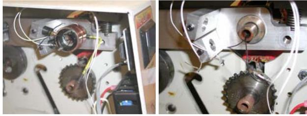
12. Remove the snap ring on the upper rear roller discard the snap ring, do not reuse the snap ring. If there are any spacers on the shaft, these must be put back in step 43.
